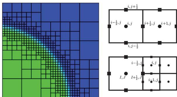
**Fig. 3** Numerical discretization: a typical spatial discretization employed during the simulations to resolve a bilayer domain (left). The Cahn–Hilliard equations are discretized using a finite volume numerical method with fluxes represented on the faces of the control volumes and the phase field  $c$  represented in the centers of the control volumes (right).
